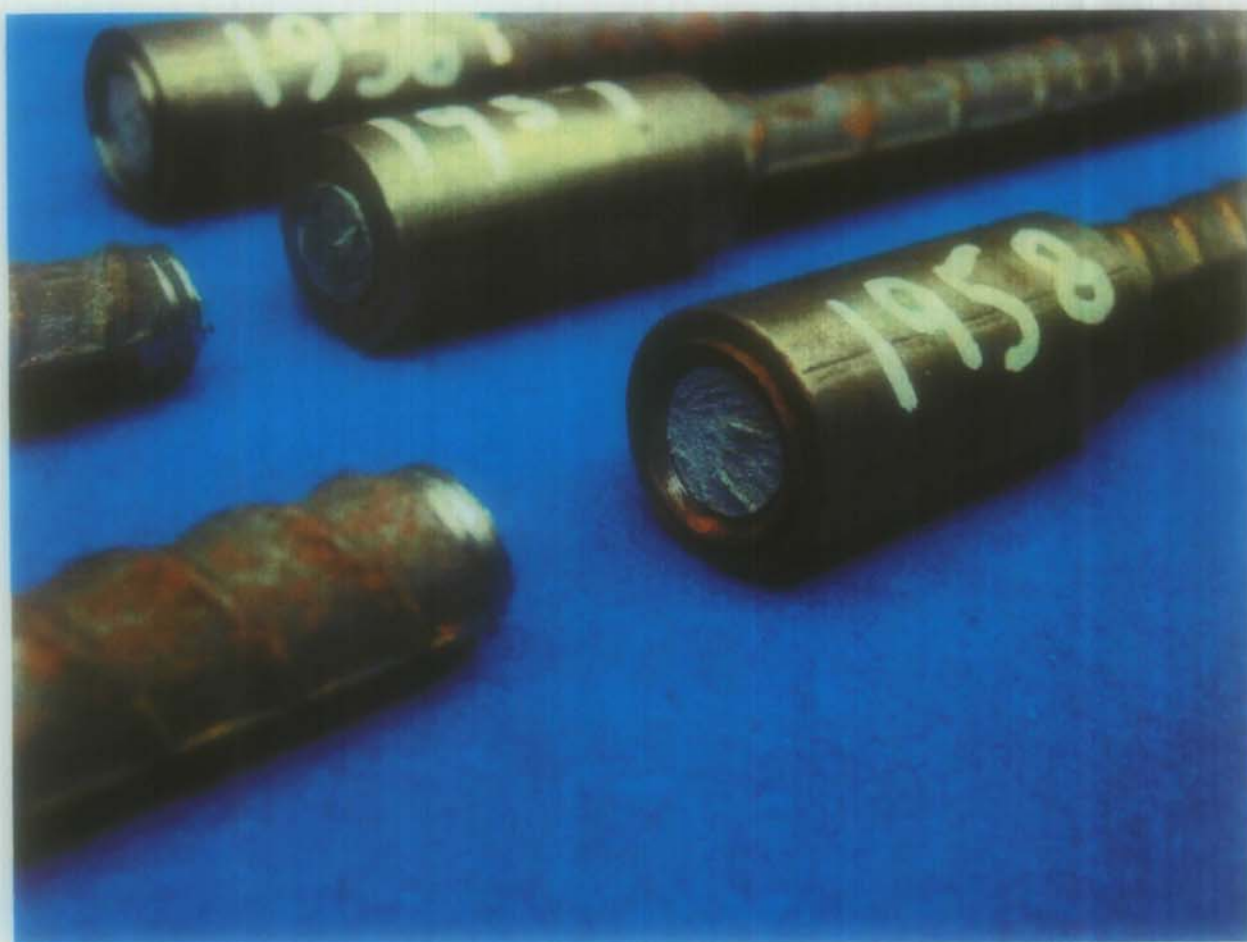
Figure 3 - Representative Fracture of Spliced Bar Specimens
